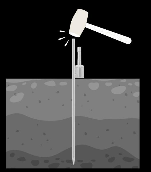
Step 1: Use a mallet/hammer to put the stake in the ground as deep as possible, or use other secure base stand.
