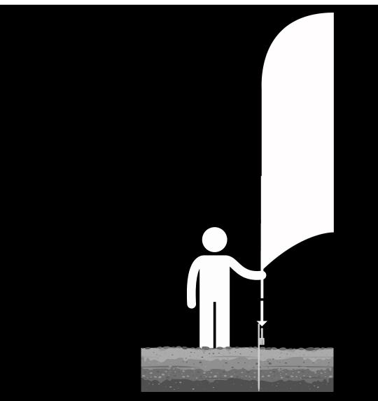
Step 3: Insert the assembled pole into the flag sleeve (sleeve size 1.6inch+), connect to the ground stake/base.
